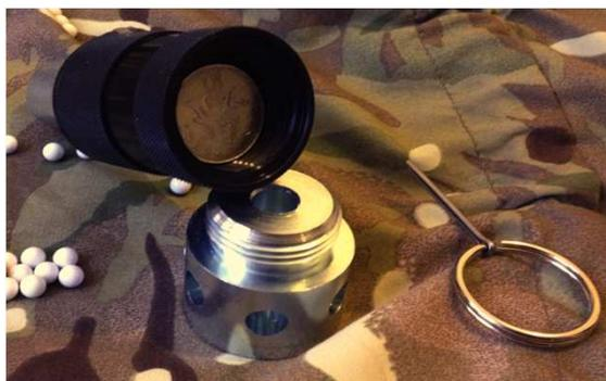
Holding the coin in position with your thumb, push down the head of the OSB SHOCK and twist the pin through the head and what we refer to as 'the wobble bit' (we couldn't think of something else to call it!) The pin should pull the wobble bit up into the head as you twist it. One side of the pin is shorter than the other to allow this to be achieved.
